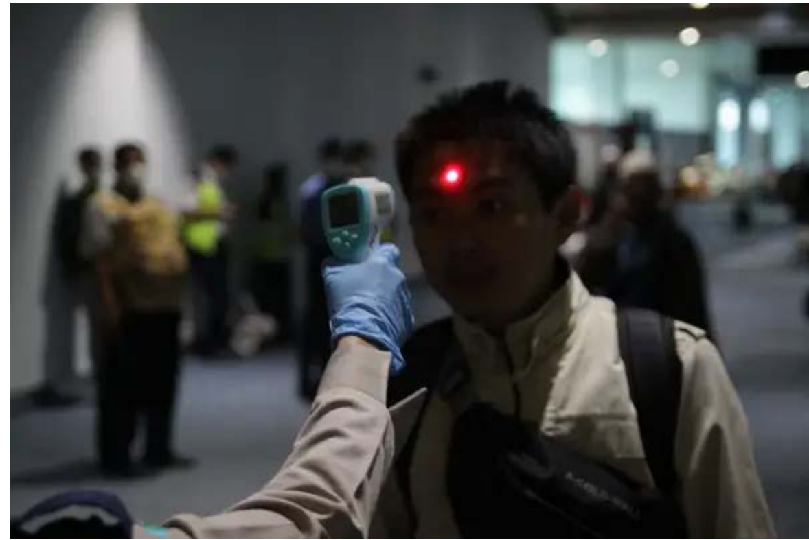
Hand-held thermometers can be unreliable due to skin temperature being colder than internal body temperature.
